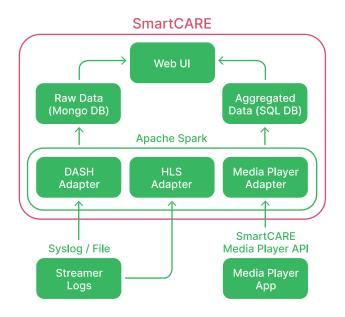
As a component of SmartTUBE solution, SmartCARE collects data on its clients, resources and streaming; access to reports is provided through the SmartTUBE administration web interface:
